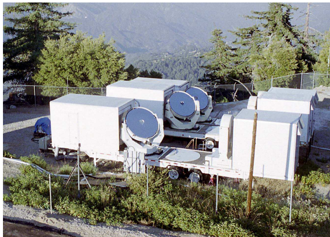
Figure 5: Mid-infrared array of three 1.65 m telescopes at Mt. Wilson, used in interferometer configuration to measure stellar diameters and their surrounding disks.
