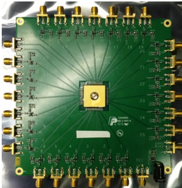
Fig. 5. The discrete amplification avalanche photodiode 5x5-pixel array developed by Amplification Technologies became available in March 2016. 10x10-pixel DA-APD arrays are slated to be available by the end of 2016. Each of the 25 SMA connectors services one of the individual pixels.
