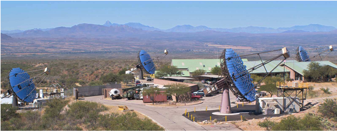
Figure 4: The Veritas array of imaging Cherenkov telescopes in Arizona consists of four 12m light buckets, each with a focal plane of 499 photo-multipliers.
